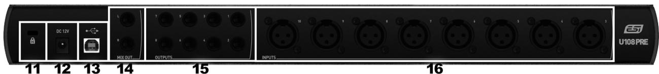
11. If required, this connects your unit to a standard **laptop lock connector**, preventing it from being stolen.
